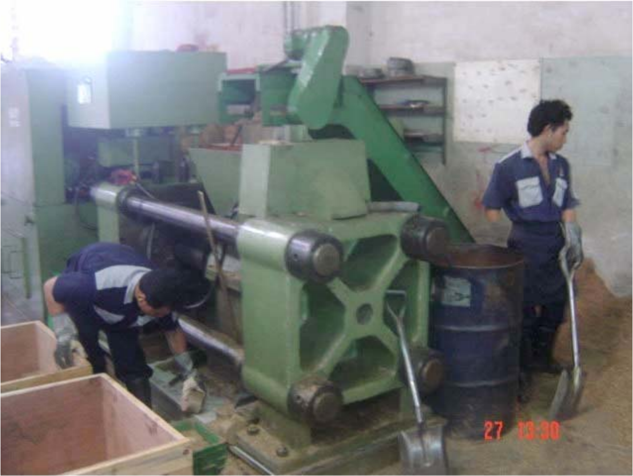
Briquetting press used at a customer's company Briquetting press used in Thailand – Brass Briquetters
